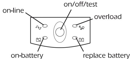
Press the **on/off/test** button with the UPS plugged in to turn the UPS on or off. See Sec. 5.1.
