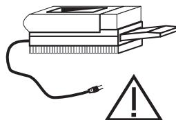
**Caution:** Do not connect a laser printer to the UPS along with other computer equipment unless the UPS is rated 1400 VA. A laser printer periodically draws significantly more power than when idle, and may overload the UPS. Verify that the UPS can support the loads when the printer is in full operation (printing).
