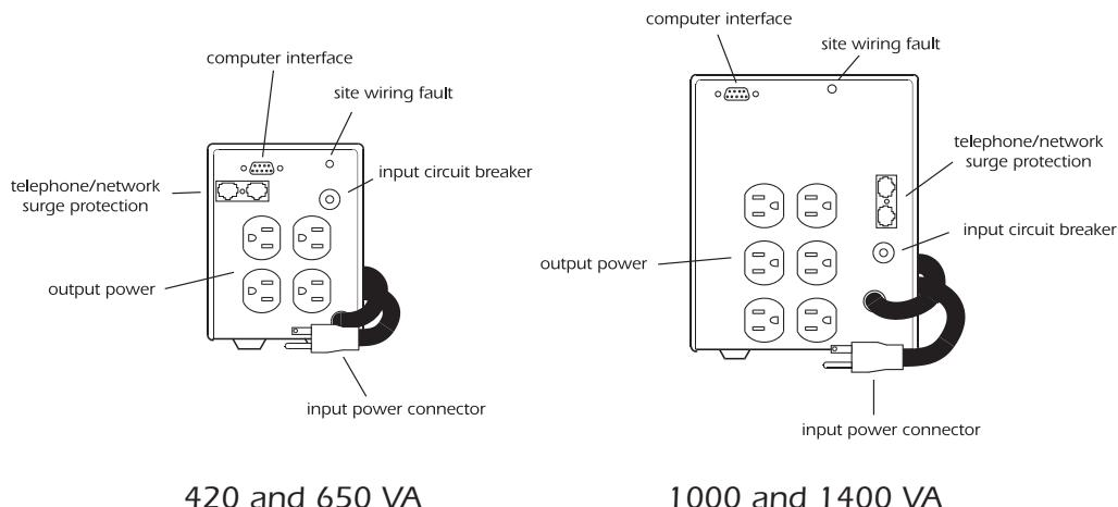
The **input power connector** is a power cord with a NEMA 5-15P connector.
