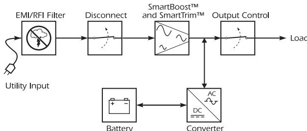
This high-performance, line-interactive, uninterruptible power source (UPS) provides clean, reliable, AC power to computer systems — protecting them from power blackouts, brownouts, swells, sags, surges, and interference.
