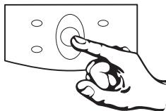
With the UPS plugged in, press the on/off/test button to supply power to the loads. The loads are immediately powered while the UPS beeps and performs a self-test. See section 5.2. Press the button again to turn off power to the loads. It may be convenient to use the UPS as a master on/off switch for the protected equipment.
