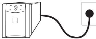
Plug the UPS into a two-pole, three-wire, grounded receptacle only. Avoid using extension cords and adapter plugs.
