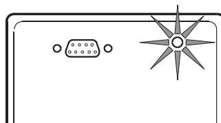
After plugging in the loads and the UPS, check the site wiring fault indicator on the rear panel. See section 3.2 for the location of the indicator on the back panel. It lights if the UPS is plugged into an improperly wired AC power outlet. Wiring faults detected include missing ground, hot-neutral polarity reversal, and overloaded neutral circuit.
