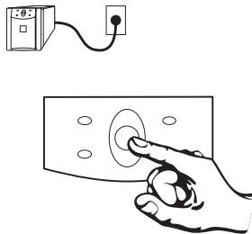
Use the self-test to verify both the operation of the UPS and the condition of the battery. With the UPS plugged in to normal utility power and turned on, activate the self-test by pressing **and bold-ing** the on/off/test button until the on-line LED flashes. This takes about 4 seconds.
