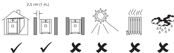
Install the UPS in a protected area with adequate air flow the areas should be free of excessive dust. Do not operate the UPS where the temperature and humidity is outside the specified limits. See section 12. Allow the UPS to come to room temperature before continuing.
