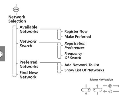
In order for the phone to make and receive phone calls, it must register with one of the available networks. These can be either GSM900, GSM1800 or combined GSM900/1800 types of network.
