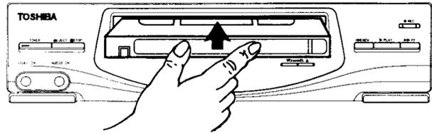
**Insert a cassette.** Push the cassette gently through the door of the cassette compartment until the VCR mechanism pulls it into the VCR. Inserting a cassette will automatically turn on the VCR's power. The cassette-in indicator (
