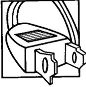
Your VCR operates on 120 volts, 60 Hz (normal household current) and has a polarized plug. Because one blade of the plug is wider than the other, the plug fits in the wall socket only one way. Do not defeat the safety feature of this plug. If you need an extension, use a polarized cord.
