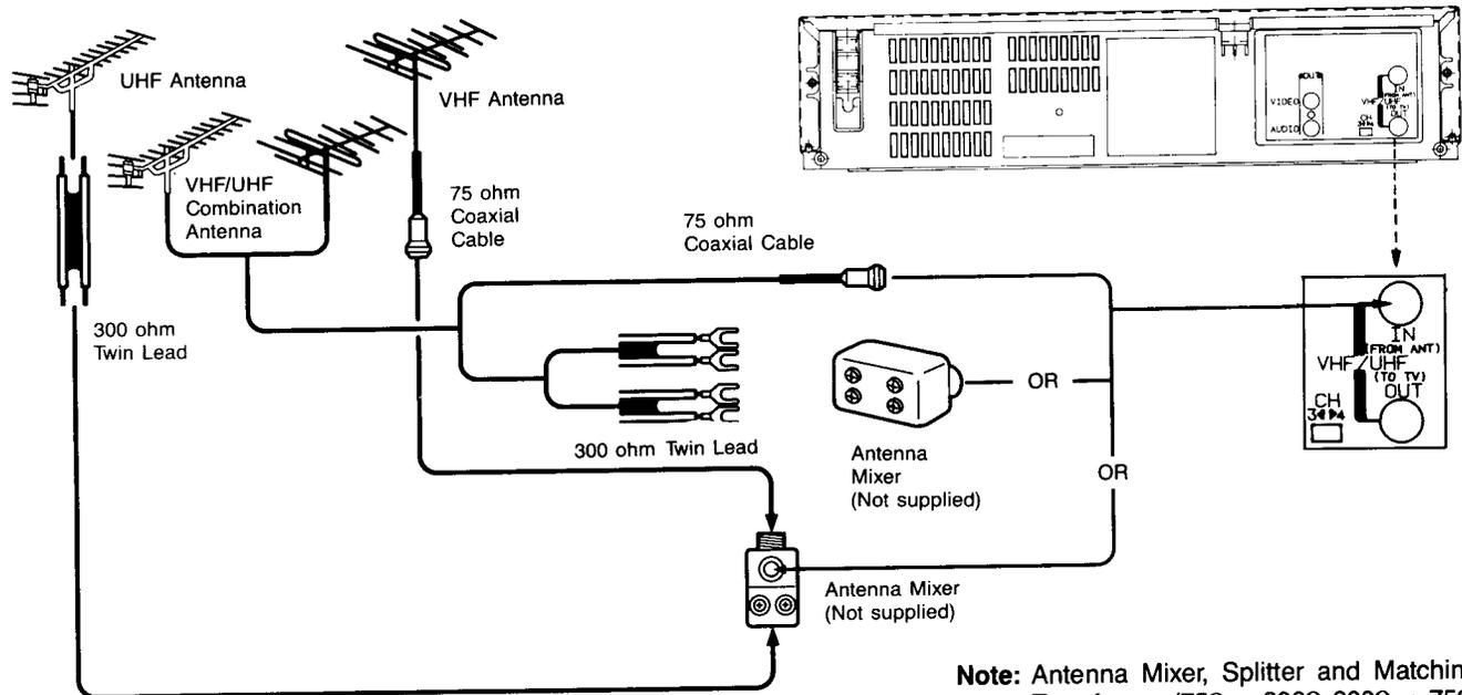
**Note:** Antenna Mixer, Splitter and Matching Transformer (75Ω ⇌ 300Ω, 300Ω ⇌ 75Ω) is available from your local electronics store.
