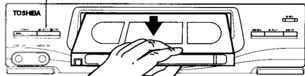
**Eject and remove a cassette.** The VCR must be in the stop mode. Press the *EJECT/STOP* button to eject the cassette. The cassette is partially ejected automatically by the VCR. Gently pull the cassette straight back out of the compartment. Place the cassette in its case and store it upright.
