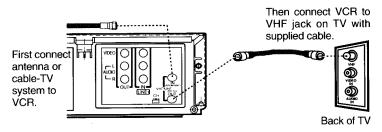
**Remember:** When you connect the *OUT TO TV* jack on the VCR to the TV as shown above, you will be tuning your TV to channel 3 or 4 to see the signals from the VCR.
