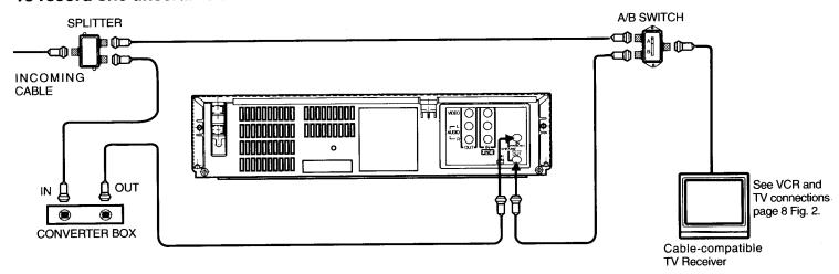
Notes: Set the VCR channel selector to output Channel of the converter.
