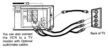
**Remember:** When you connect the *AUDIO* and *VIDEO OUT* jacks on the VCR to a TV monitor as shown above, you will be tuning your monitor to its video input channel (varies with TV models) to see the signal coming from the VCR. You will also be able to see the VCR's signal on channel 3 or 4.
