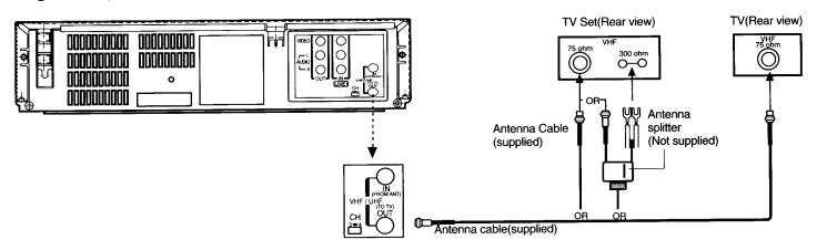
Fig. 2 VHF/UHF(75ohm/300ohm) or VHF/UHF(75ohm) terminals connection
