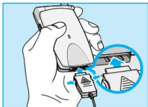
1. Insert one end of the travel adapter into the bottom of the phone.
