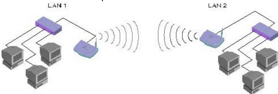
Wireless Bridge Point-to-Point mode
