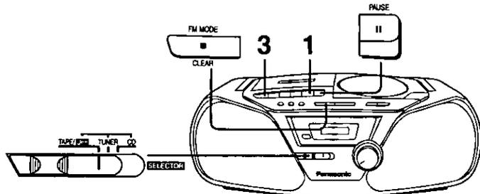
**1** Press [STOP/EJECT] to open the tape lid and load the tape. Close the tape lid by hand.
