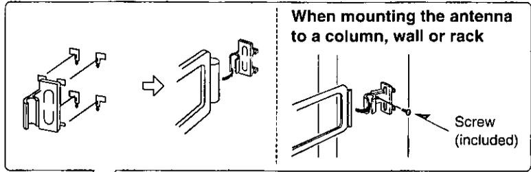
When mounting the antenna to a column, wall or rack
