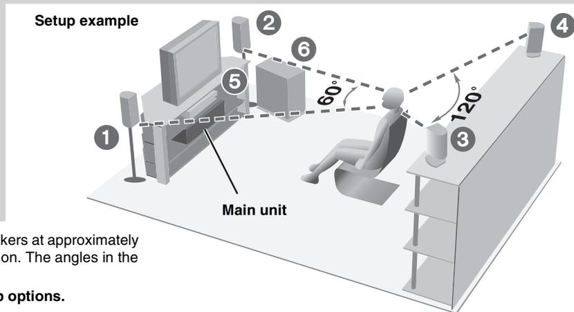
Place the front, center and surround speakers at approximately the same distance from the seating position. The angles in the diagram are approximate.
