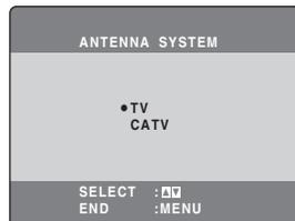
Channels are set corresponding to the antenna system you select. This is set automatically when you do Plug-in Auto Tuning.
