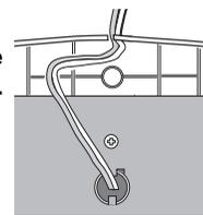
B Press the speaker cable against the base while threading it between the pegs.
