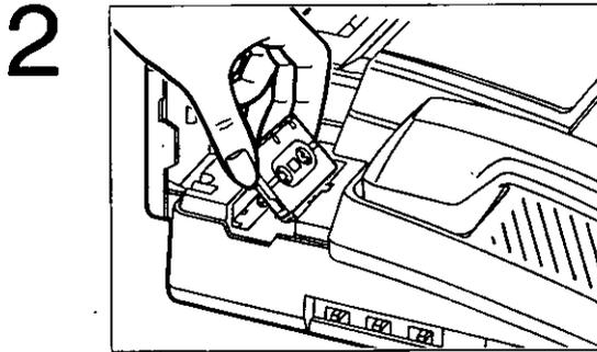
Insert the microcassette tape into the compartment with the full reel to the left. Make sure that there is no slack in the tape. Remove any slack by using a pencil and rotating the tape reel.
