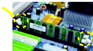
Fig.2 Close the plastic clip at both edges of the DIMM sockets to lock the DIMM module. Reverse the installation steps when you wish to remove the DIMM module.
