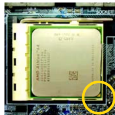
Fig.2 A gold-colored triangle is marked one edge of the CPU. Please align this edge with the socket edge closest to the CPU lever. Gently place the CPU into position making sure that the CPU pins fit perfectly into their holes. Once the CPU is positioned into it socket, place one finger down on the middle of the CPU and gently press the metal lever back into its original position.
