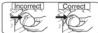
① Align the Key of the bottle, also represented by the Arrow mark (**Unlocked** symbol 🗝️) visible on the end of the Toner Bottle with the Arrow mark on the machine.
