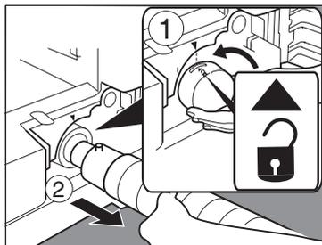
① Turn the empty Toner Bottle counter-clockwise until it stops. The Arrow mark (**Unlocked** symbol
