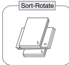
Multiple copies sorted automatically and Stacked in alternate direction.
