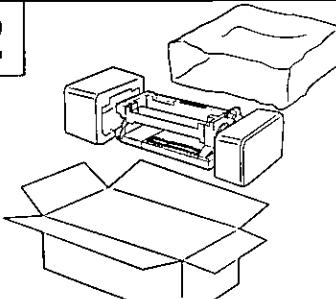
Remove the new fuser from its packaging; keep the fuser upright.
