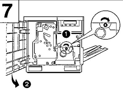
① Turn the small green thumbscrew clockwise to lock the fuser.
