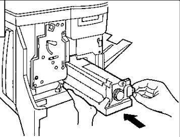
Insert the new fuser into the printer.
