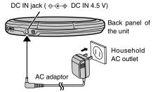
Recharging starts. The main unit's recharging lamp (CHG) lights and the battery indicator on the remote control scrolls.
