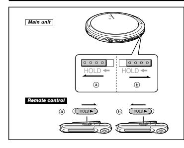
This function causes the unit to ignore short, accidental button presses. (The disc lid can still be opened and closed.)
