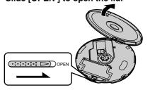
2 Open the battery lid and insert the two rechargeable batteries. Press to open in step ().
