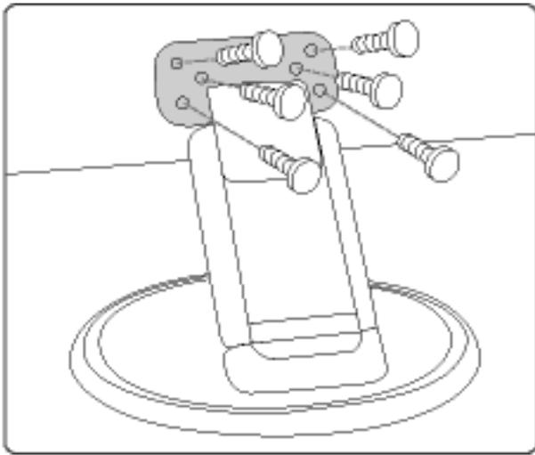
**2)** Remove the 6 screws and then remove the base from the LCD monitor.
