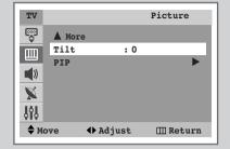
If you find that the picture received is slightly tilted to one side, you can adjust the tilt setting.
