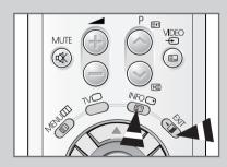
You can set the television's clock so that the current time is displayed by pressing the "INFO ()" button. You must also set the time if you wish to use the automatic on or off timers.
