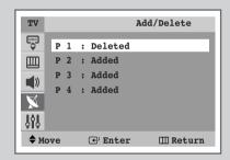
You can exclude the channels you chosen from the channels you scanned. When you scan through the stored channels, those you have chosen to skip are not displayed.
