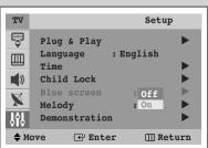
If no signal is being received or the signal is very weak, a blue screen automatically replaces the noisy picture background.
