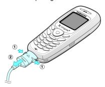
**Note:** You must unplug the adapter before you remove the battery from the phone during charging; otherwise, the phone could be damaged.
