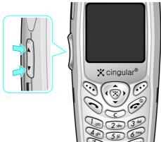
In Idle mode, you can also adjust the keypad tone volume using these keys.
