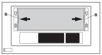
You should take out the metal filter every four weeks and wash it either in the dishwashing machine or by hand.
