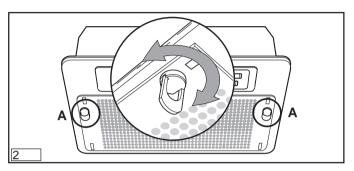
2) Unscrew the lamps that do not work and replace them with 40W max lamps (E14).
