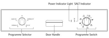
Set the point at which the wash programme is to start using the **pro-gramme switch**. The programme switch rotates during the wash programme and indicates the position that has been reached in the programme.
