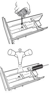
7. Use a brush to clean the entire compartment area of the washing machine, particularly also the nozzles on the top side of the compartment.
