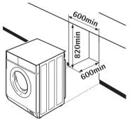
(Measurements in mm)
