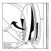
Fluff is more easily removed if you damp your hand slightly or use a damp cloth. After cleaning the fine filter, fold down and clip in coarse filter.
