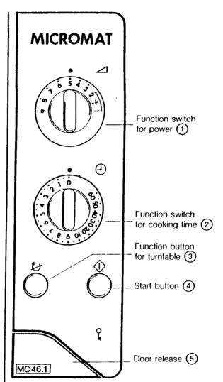
Place mains plug in socket with protective earth contact. Press door release **5** %, open door, insert food, and close door.
