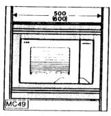
Caution! When installing the MICROMAT model 120 behind a roller door, the door must always be open when the oven is in use.
