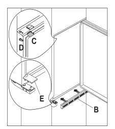
Snap vent grill (B) and hinge cover (E) into position.
