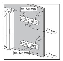
6. Place guide (Ha) on the inside part of the furniture door, up and down as shown in the figure and mark the position of external holes. After having drilled holes, fix the guide with the screws supplied.
