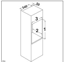
It is necessary that the cabinet has a ventilation recess with the following dimensions: Depth 50 mm Width 540 mm
