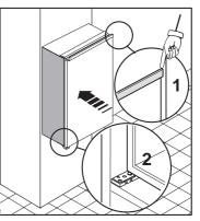
1. Fit the appliance in the niche by making sure that it stands against the interior surface of the unit on the side where the door hinges of the appliances are fitted. Insert the appliance until the upper strip butts up against the unit (1) and make sure that the lower hinge is in line with the surface of the unit (2).
