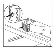
press on the rear hook and at the same time slide the cover in the direction indicated by the arrow.
