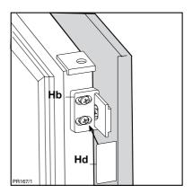
If the appliance is fixed to the side of the kitchen unit, simply slacken the screws in fixing brackets (E), move the brackets as shown in the figure and retighten the screws.
