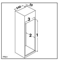
Fit the appliance in the niche by making sure that it stands against the interior surface of the unit on the side where the door hinges of the appliances are fitted. Insert the appliance until the upper strip butts up against the unit (I) and make sure that the lower hinge is in line with the surface of the unit (2).
