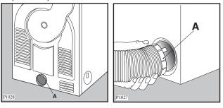
Advice: If the hose is long and the room temperature low, the moisture might condense to water inside the hose. This is nothing to be concerned about. To prevent this water from lying in the hose or flowing back into the tumble dryer, it is advisable to drill a small hole (dia. 3 mm) in the lowest point of the hose and to place a small container below it.(See picture, point B).
