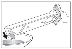
Slide the outlet connections in and refit the water reservoir. If the programme has been interrupted as
