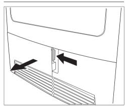
Open door in plinth: To do this, press the release button on the right and open the door in the plinth to the left.
