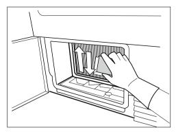
As necessary, approx. once every 6 months, remove the fluff from the heat exchanger using the sponge supplied. When doing this, please use rubber gloves.
