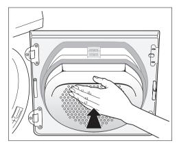
**1** If the fine filter is not fitted, the large mesh filter will not snap into place and the loading door cannot be closed.
