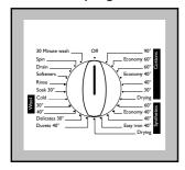
The selector dial can be turned either clockwise or anticlockwise to select the required wash and drying programme .
