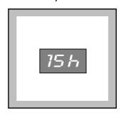
The delay time is displayed for 3 seconds, then the duration of the selected programme reappears.
