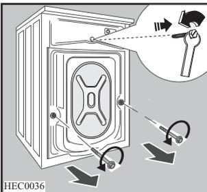
Slide out the relevant plastic spacers. Open the porthole and remove the polystyrene block fitted on the door seal.
