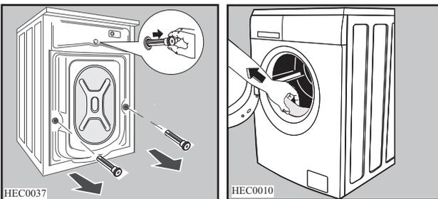
Fill the smaller upper hole and the two large ones with the corresponding plastic plug caps supplied in the bag containing the instruction booklet.
