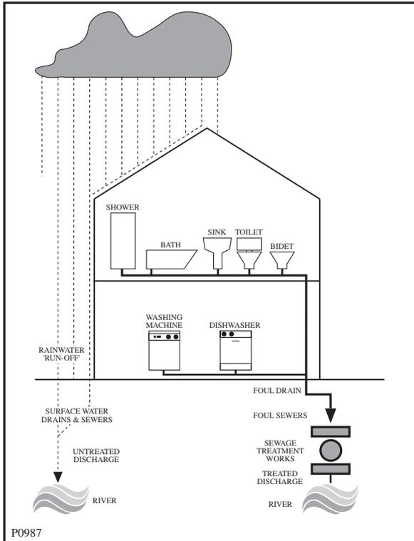
It is essential that these appliances are not connected to the surface water drainage system as this water is discharged directly into a river or stream and may cause pollution. If you require any further advice please contact your local water authority.
